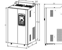
15-220kW (Iron shell) support Wall-Hang Installation and Flange installation
