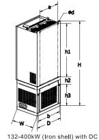
132-400kW (Iron shell) with DC reactor base and Floor Installation
