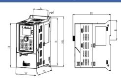
0.75-4kW (plastic shell) support Guide rail installation
