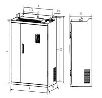
250-400kW ( Iron shell)support Wall-Hang Installation and Floor Installation
