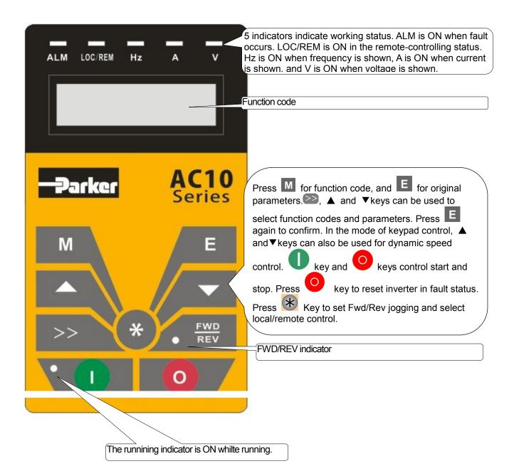
Figure 5-1 Keypad Displays
